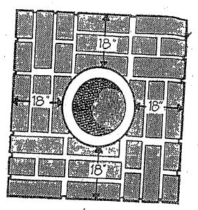
THIMBLE OR CONNECTOR THROUGH COMBUSTIBLE WALL (MINIMUM 18" AIRSPACE OR NONCOMBUSTIBLE MATERIAL AROUND THIMBLE OR CONNECTO
